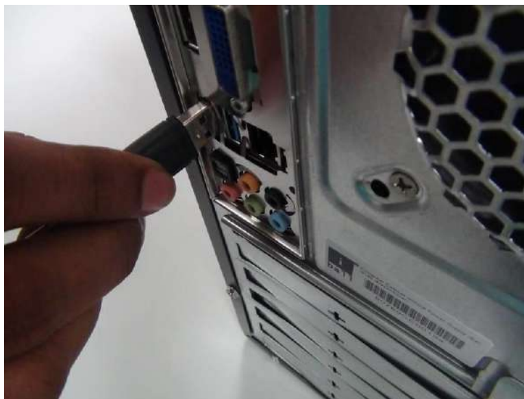
Figure 8: Connecting USB Type-A to Type-C Cable to SuperSpeed Port
