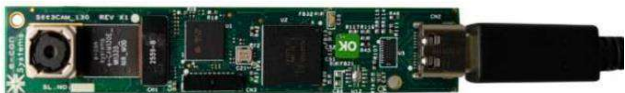
Figure 5: USB Type-A to Type-C Cable inserted in USB Type-C Connector
