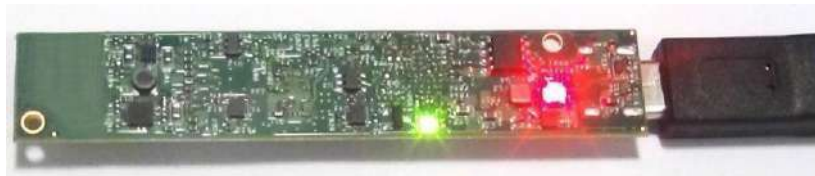
Figure 10: Status LED indicating Camera Streaming
